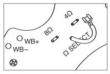
Figure 15 Setting the Impedance Jumper.
